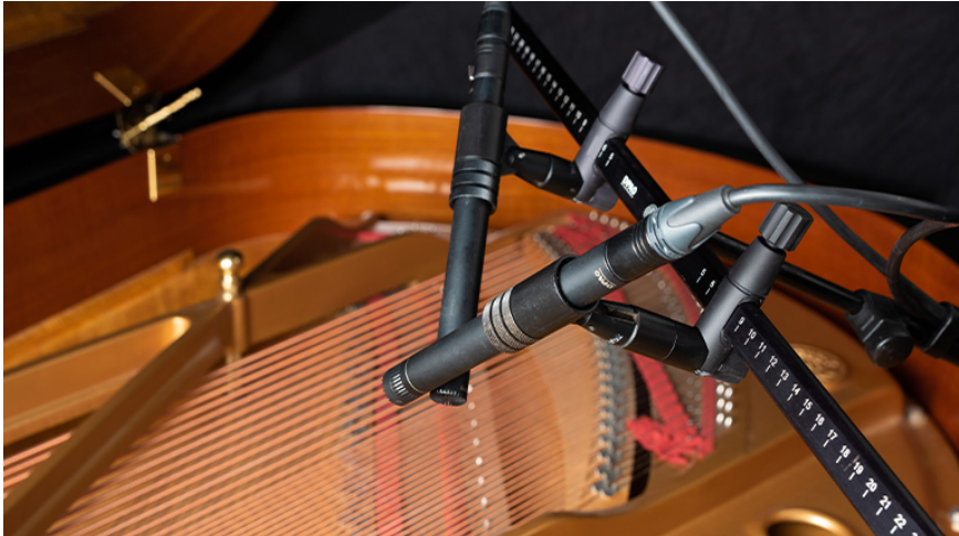
Fig. 9 Mounting the microphones closely but without any physical contact.
