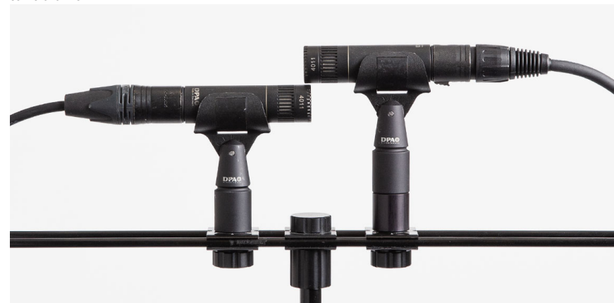
Fig. 13 Here, two cardioids replace a figure-of-eight microphone. Two microphone inputs are needed in principle. However, you can "cheat" by using a Y-sum cable with pin 2 and 3 reversed in one microphone connector.
